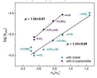
Fig. 2 (a) LFER analysis varying the aryl fluoride, correlated with  $\sigma_X^-$ . (b) A different analysis of the same data, using  $\sigma_X$  for  $-4-\text{CF}_3$  and -4-COMe. In both plots,  $\sigma$  values were used for substituents with either no  $\sigma^-$  value or a nearly identical  $\sigma^-$  value. Indole (Y = H) and 5-cyanoindole (Y = CN) were used as the nucleophiles.
