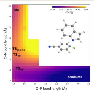
Fig. 7 Calculated potential energy surface for the anionic reaction, showing a borderline mechanism. The predicted geometries for the anionic transition state,  $TS_{SB}$ , and  $TS_{G}B$  are marked. Calculations carried out at B3LYP-D3(BJ)/6-31+q\*/CPCM(DMF).
