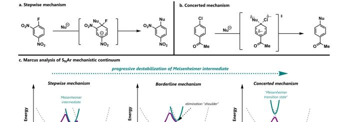
Scheme 1 (a) A representative stepwise  $S_NAr$  reaction with a highly activated electrophile and poor leaving group. (b) A representative concerted  $S_NAr$  reaction with a less activated electrophile and better leaving group. (c) A qualitative Marcus analysis applied to  $S_NAr$  mechanisms.
