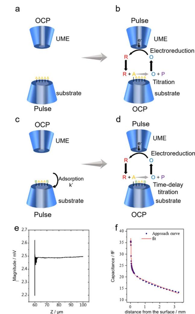
Fig. 1 (a–d) Schematic diagrams of SECM operation in SI mode. P represents the byproduct of the reaction between R and A. B is a substance that competes with A for adsorption on the substrate. (e) Shear force based approach curve. Reproduced with permission from ref. 69, Royal Society of Chemistry, 2021. (f) Capacitive approach curve obtained (blue circles) with its fit to the theoretical result (red line). Reproduced with permission from ref. 71, American Chemical Society, 2019.
