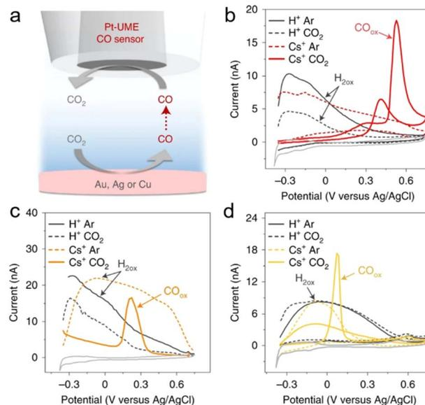
Fig. 7 (a) Schematic representation of the SECM experiment. (b) CV on the Pt UME obtained directly after  $\text{CO}_2$  reduction on gold electrodes. (c) CV on the Pt UME obtained directly after  $\text{CO}_2$  reduction on silver electrodes. (d) CV on the Pt UME obtained directly after  $\text{CO}_2$  reduction on copper electrodes. The CVs on the Pt-UME before applying any potential to the sample are shown in light grey for reference. Reproduced with permission from ref. 111, Nature, 2021.
