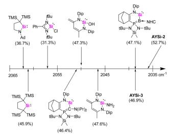
Fig. 4 Comparison of the TEP values for various silylenes determined by asymmetric CO stretching frequency of LNi(CO)<sub>3</sub> in toluene at room temperature.  $^{26.31}$  %  $V_{\rm bur}$  is given in parentheses.
