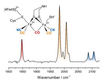
Fig. 1 Schematic representation and linear IR absorption spectrum of the H-cluster in the  $H_{inact}$  state. The IR spectrum was recorded from DdHvdAB.
