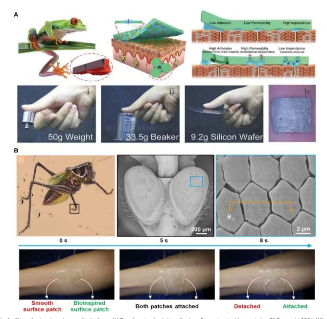
Fig. 8 Skin adhesives based on capillarity force. (A) Tree frog-inspired skin adhesives. Reproduced with permission.<sup>110</sup> Copyright 2024, Wiley-VCH. (B) Chinese cricket-inspired skin adhesives. Reproduced with permission.<sup>111</sup> Copyright 2023, AAAS.
