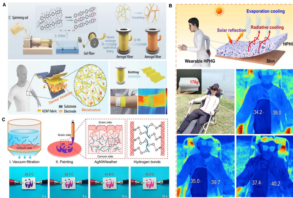
Fig. 9 Skin adhesive for wearable thermal management devices. (A) Photos and device structures of polymer aerogel fibers for passive thermal management. Reproduced with permission. 130 Copyright 2024, Elsevier. (B) Silver nanowire decorated leather with hierarchical structures for integrated visual Joule heating. Reproduced with permission. 131 Copyright 2022, Wiley-VCH. (C) Schematic illustration of textiles based on zylon aerogel fibers for self-powered sensing in harsh environments. Reproduced with permission. 132 Copyright 2024, Wiley-VCH.
