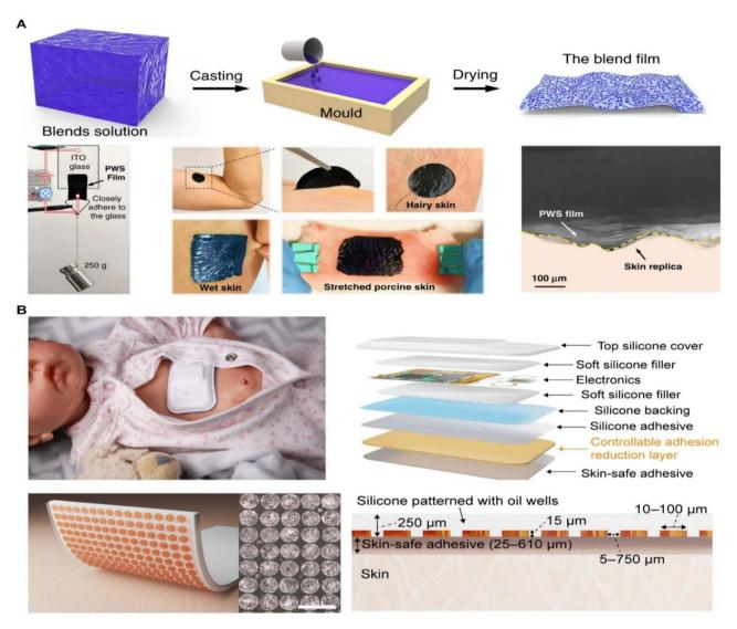
Fig. 6 Skin adhesives based on Films and Elastomers. (A) Film-based skin adhesives. Reproduced with permission.<sup>97</sup> Copyright 2020, Springer Nature. (B) Elastomers-based skin adhesives. Reproduced with permission.<sup>98</sup> Copyright 2022, AAAS.
