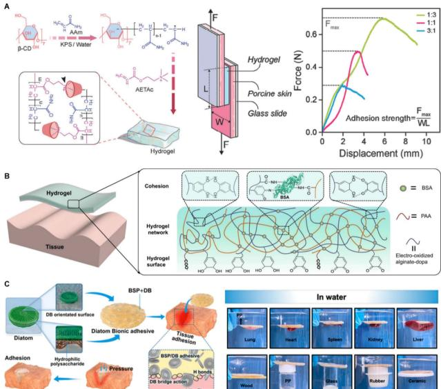
Fig. 5 Skin adhesives based on hydrogel. (A) Synthetic hydrogel-based skin adhesives. Reproduced with permission.<sup>83</sup> Copyright 2024, Wiley. (B) Protein hydrogel-based skin adhesives. Reproduced with permission.<sup>84</sup> Copyright 2021, AAAS. (C) Polysaccharide hydrogel-based skin adhesives. Reproduced with permission.<sup>85</sup> Copyright 2023, ACS.
