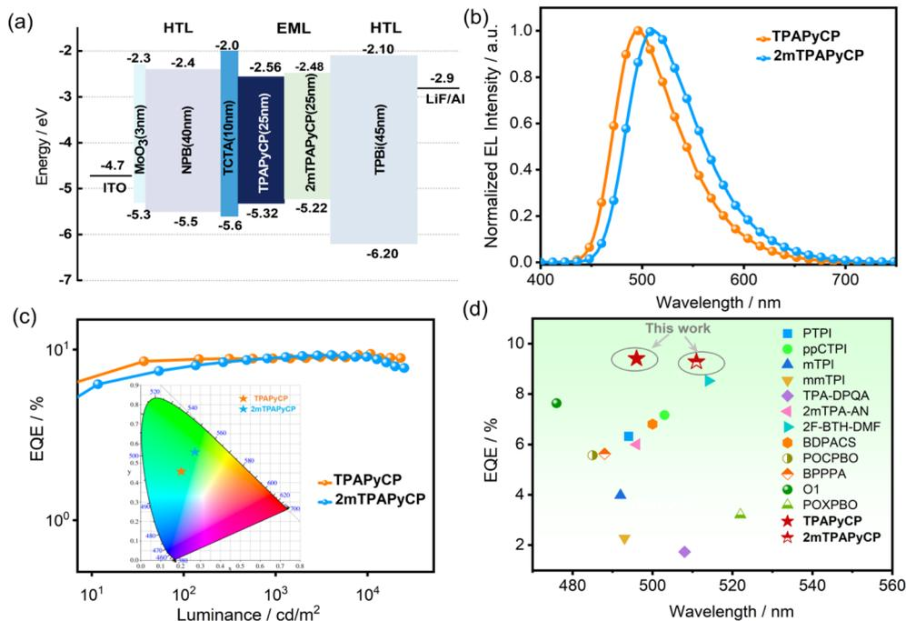
Fig. 4 (a) Device structure and energy diagram; (b) EL spectra under a voltage of 5 V; (c) EQE versus luminance curves; insert: corresponding CIE coordinates for the devices, (d) the reported maximum EQE based on hot-exciton materials with the EL emission peaks in the range of 470–520 nm.
