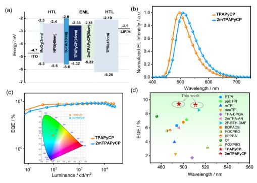
Fig. 4 (a) Device structure and energy diagram; (b) EL spectra under a voltage of 5 V; (c) EQE *versus* luminance curves; insert: corresponding CIE coordinates for the devices, (d) the reported maximum EQE based on hot-exciton materials with the EL emission peaks in the range of 470–520 nm.
