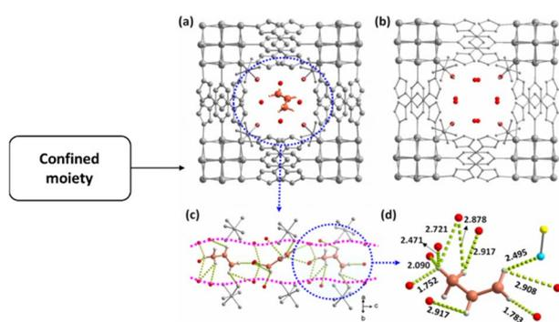
Fig. 11 Crystal structure of loaded C<sub>3</sub>H<sub>6</sub> and C<sub>3</sub>H<sub>8</sub> samples: (a) NTU-85-WNT@C<sub>3</sub>H<sub>6</sub> and (b) NTU-85-WNT@C<sub>3</sub>H<sub>8</sub> and (c, d) detailed H-bonding interactions of C<sub>3</sub>H<sub>6</sub> in one-dimensional nanochannels. Reprinted with permission from ref. 37. Copyright 2023 American Chemical Society.
