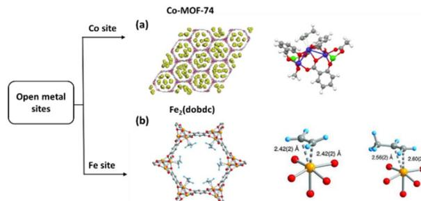
Fig. 2 (a) A snapshot from a GCMC simulation for  $C_3H_6$  adsorption in Co-MOF-74, and the propylene molecule binds to the Co atom. (b) A portion of the solid-state structure of  $Fe_2(dobdc) \cdot 2C_2D_4$ , and  $C_2H_4$ , and  $C_3H_6$  coordination with  $Fe_2(dobdc)$ . Reprinted with permission from ref. 22. Copyright 2012 John Wiley & Sons, ref. 31. Copyright 2012 The American Association for the Advancement of Science, respectively.
