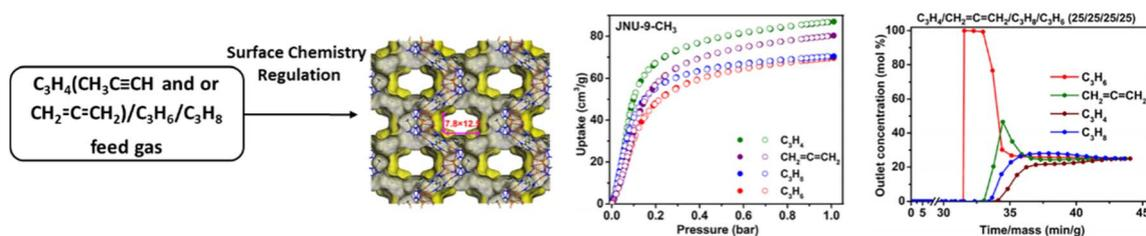
Fig. 22 The crystal structure of JNU-9-CH<sub>3</sub>, adsorption isotherms for C<sub>3</sub>H<sub>4</sub>, CH<sub>2</sub>=C=CH<sub>2</sub>, C<sub>3</sub>H<sub>6</sub> and C<sub>3</sub>H<sub>8</sub> at 298 K, and breakthrough experimental curves of C<sub>3</sub>H<sub>4</sub>, CH<sub>2</sub>=C=CH<sub>2</sub>, C<sub>3</sub>H<sub>6</sub> and C<sub>3</sub>H<sub>8</sub> (25/25/25/25, v/v/v) mixtures at 298 K. Reprinted with permission from ref. 60. Copyright 2024 American Chemical Society.
