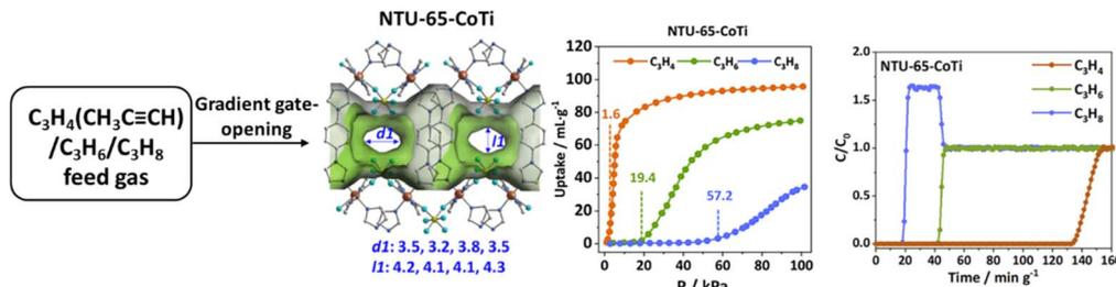
Fig. 19 The crystal structure of NTU-65-CoTi, adsorption isotherms for  $C_3H_4$ ,  $C_3H_6$  and  $C_3H_8$  at 273 K, and breakthrough experimental curves of  $C_3H_4/C_3H_6/C_3H_8$  (0.5/49.75/49.75, v/v/v, 2 mL min<sup>-1</sup>) mixtures at 273 K. Reprinted with permission from ref. 51. Copyright 2024 The Royal Society of Chemistry.
