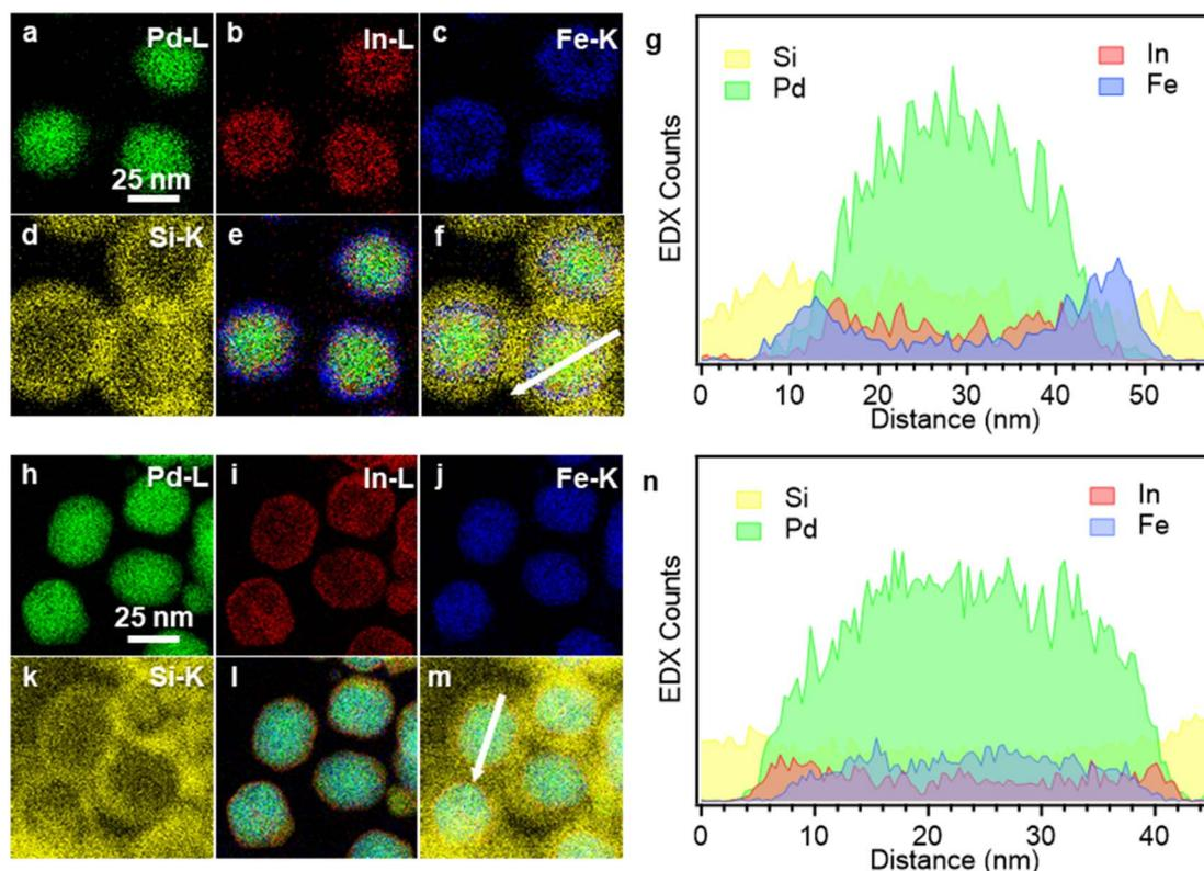
Fig. 2 (a–d and h–k) EDX elemental maps (Pd-L (a and h), In-L (b and i), Fe-K (c and j) and Si-K (d and k)) of  $\text{FePd}_3\text{:In}$  (a–d) and  $\text{PdIn}_x\text{:Fe}$  (h–k) NPs. (e, f, l and m) Overlay of a–c (e), (a–d) (f), h–j (l) and (h–k) (m). (g and n) EDX line profiles indicated by the white arrows in f and m.
