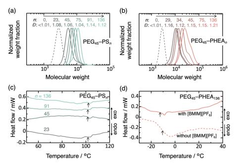
Fig. 1 SEC traces (a and b) and DSC thermograms (c and d) of  $PEG_{45}-PS_n$  (a and c) and  $PEG_{45}-PHEA_n$  (b and d). DSC was performed with the non-volatile solvent [BMIM][PF<sub>6</sub>] present, at the polymer concentration of 40 wt%, except for the dotted curve in panel (d). Arrows in panels (c) and (d) indicate  $T_g$ . In panels (a) and (b), "molecular weight" represents the relative molecular weight obtained with poly(methyl methacrylate) standards.
