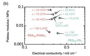
Fig. 5 (a) Quasi-phase diagram of  $PEG_{45}-PS_n$  (high- $T_g$  core-forming block) and  $PEG_{45}-PHEA_n$  (low- $T_g$  core-forming block) prepared via PISA in [BMIM][PF<sub>6</sub>] in 40 wt% solute. (b) Plateau modulus obtained from oscillatory rheometry plotted against electrical conductivity for  $PEG_{45}-PS_n$  (turquoise symbols) and  $PEG_{45}-PHEA_n$  (pink symbols) in [BMIM][PF<sub>6</sub>] with 40 wt% solute at 25 °C.
