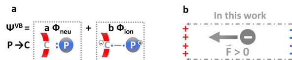
Scheme 1 (a) Illustration of the complete VB wavefunction with two Lewis (resonance) structures; (b) definition of the electric field direction in this work.
