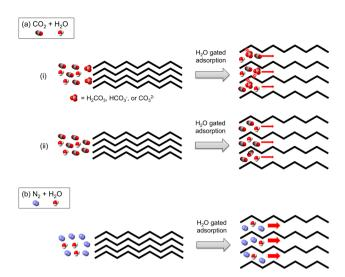
Fig. 7 Possible source of the coexisting gas dependency of the  $H_2O$  adsorption rate. (a) Temporary formation of  $H_2CO_3/HCO_3^{-}/CO_3^{2^{-}}$  (i) and temporary occupancy of  $CO_2$  and  $H_2O$  in the pores (ii) under humid  $CO_2$  flow conditions. (b) Temporary occupancy of  $N_2$  and  $H_2O$  in the pores under wet  $N_2$  flow conditions.
