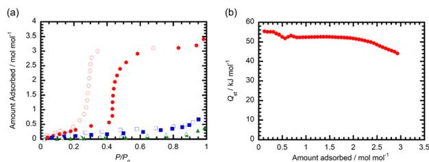
Fig. 4 (a) H<sub>2</sub>O (red circles, 298 K), MeOH (blue squares, 288 K), and EtOH (green triangle, 298 K) adsorption (filled symbols)/desorption (open symbols) isotherms of **1**. (b) Isothermic heat of water adsorption for **1**.
