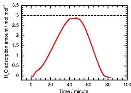
Fig. 5 Time dependence of the amount of H<sub>2</sub>O adsorbed by **1** under humidified N<sub>2</sub> (0–46 min) and dry N<sub>2</sub> (46–83 min) at 300 K.
