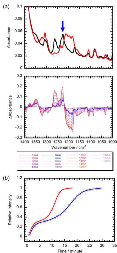
Fig. 6 (a) ATR-IR spectra of **1** (red) and **1**·3H<sub>2</sub>O (black) and difference IR spectra of **1** under wet N<sub>2</sub> at 303 K over 1 min intervals with the humid N<sub>2</sub> gas flow beginning at 0 min. (b) Time dependence of relative intensity for a peak at 1227 cm<sup>-1</sup> (blue arrow in (a) indicates the wavenumber monitored) under humid N<sub>2</sub> (red) and humid CO<sub>2</sub> (blue) at 303 K in **1**.
