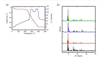
Fig. 2 (a) TG (red)-DTA (blue) curves of  $1\cdot 3H_2O$ . (b) Simulated PXRD pattern of  $1\cdot 3H_2O$  (black), observed PXRD patterns of as-synthesized  $1\cdot 3H_2O$  (red), 1 obtained after heating of  $1\cdot 3H_2O$  at 100 °C under vacuum (blue), and  $1\cdot 3H_2O$  obtained after  $H_2O$  exposure to dehydrated 1 (green).
