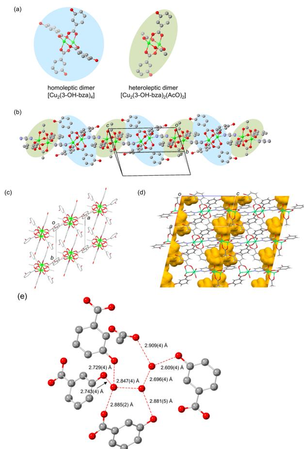
**Fig. 1** Crystal structure of **1**·3H<sub>2</sub>O. (a) Two types of contributing paddlewheel dimers forming (b) a 1D zigzag chain structure. (c) Packing of the chains, (d) one-dimensional channel structure, and (e) hydrogen bonds involving guest water molecules. The green, blue, gray, and red represent copper, nitrogen, carbon, and oxygen, respectively. Hydrogen atoms are omitted for clarity except in (d). Red dashed lines represent hydrogen bonds.
