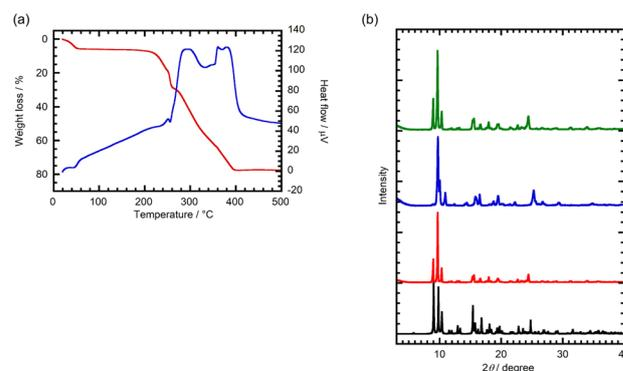
Fig. 2 (a) TG (red)-DTA (blue) curves of **1**·3H<sub>2</sub>O. (b) Simulated PXRD pattern of **1**·3H<sub>2</sub>O (black), observed PXRD patterns of as-synthesized **1**·3H<sub>2</sub>O (red), **1** obtained after heating of **1**·3H<sub>2</sub>O at 100 °C under vacuum (blue), and **1**·3H<sub>2</sub>O obtained after H<sub>2</sub>O exposure to dehydrated **1** (green).
