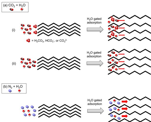
Fig. 7 Possible source of the coexisting gas dependency of the H<sub>2</sub>O adsorption rate. (a) Temporary formation of H<sub>2</sub>CO<sub>3</sub>/HCO<sub>3</sub><sup>-</sup>/CO<sub>3</sub><sup>2-</sup> (i) and temporary occupancy of CO<sub>2</sub> and H<sub>2</sub>O in the pores (ii) under humid CO<sub>2</sub> flow conditions. (b) Temporary occupancy of N<sub>2</sub> and H<sub>2</sub>O in the pores under wet N<sub>2</sub> flow conditions.
