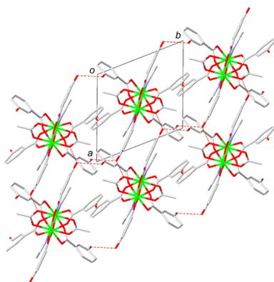
Fig. 3 EDA-derived packing structure of chains in dehydrated **1**. The green, blue, grey, and red colors represent copper, nitrogen, carbon, and oxygen, respectively. Hydrogen atoms are omitted for clarity. Red dashed lines represent hydrogen bonds.
