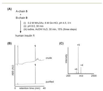
Fig. 4 Folding of native insulin: (A) reaction scheme. (B) HPLC monitoring. (C) Direct infusion analysis of purified insulin 1.
