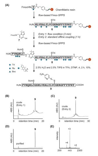
Fig. 3 (A) Synthetic scheme of insulin B-chain 9. (B)–(D) HPLC monitoring. (E) Direct infusion data of purified peptide 9.
