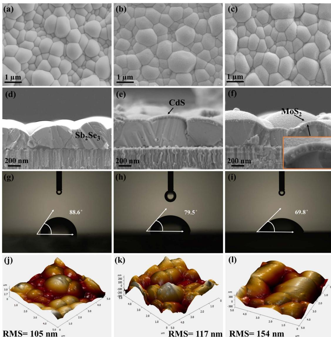
Fig. 3 SEM micrographs of (a)  $\text{Sb}_2\text{Se}_3$ , (b)  $\text{Sb}_2\text{Se}_3/\text{CdS}$ , and (c)  $\text{Sb}_2\text{Se}_3/\text{CdS}/\text{MoS}_2$  samples. (d–f) The corresponding cross-sectional SEM images. (g–i) The measured CAs (using  $\text{H}_2\text{SO}_4$  electrolyte droplets) of the samples, and (j–l) AFM images of the sample surfaces.
