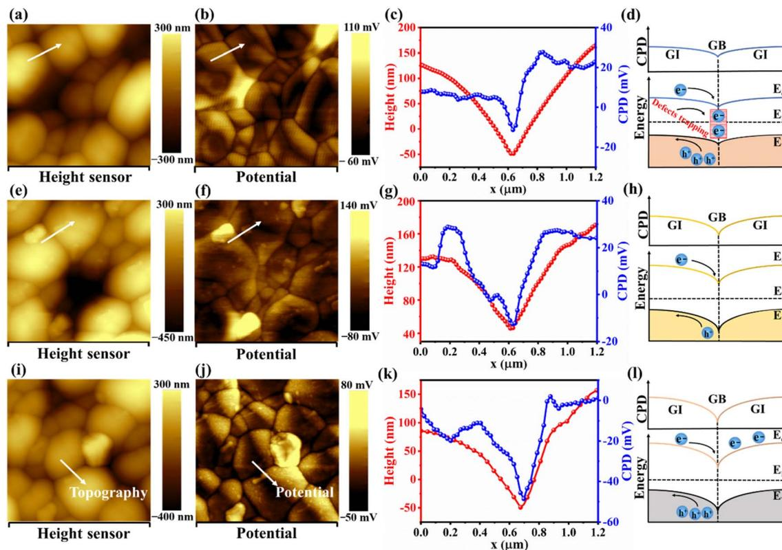
Fig. 4 KPFM scanning surface topography and CPD maps for (a and b)  $Sb_2Se_3$ , (e and f)  $Sb_2Se_3/CdS$ , and (i and j)  $Sb_2Se_3/CdS/MoS_2$  samples, respectively. (c, g and k) The corresponding topography and potential line scans acquired from the white arrow lines. (d, h and l) Schematic of the energy band structure and CPD near the GBs, where “e<sup>-</sup>” represents electrons; “h<sup>+</sup>” represents holes.
