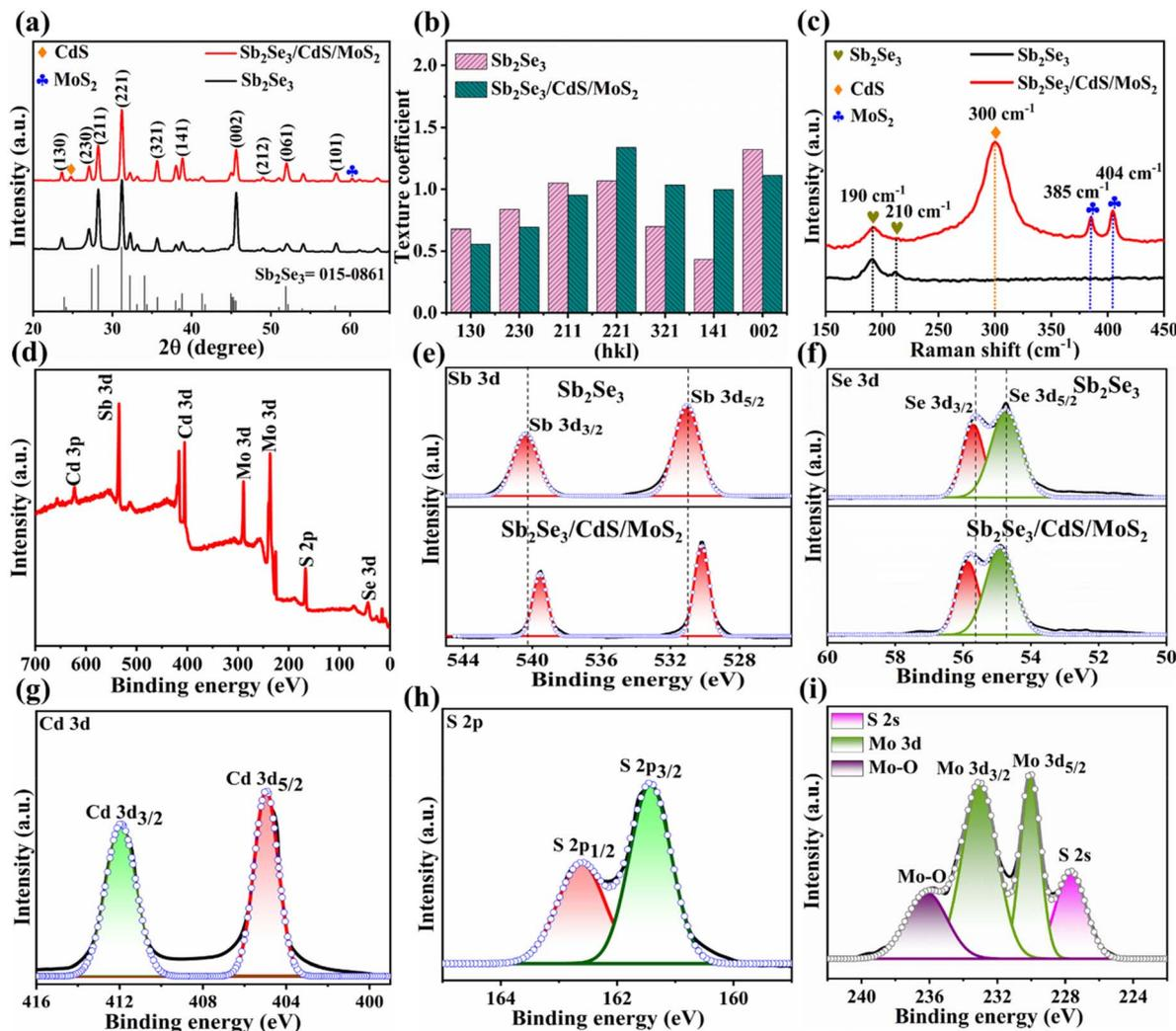
Fig. 2 (a) XRD, (b) texture coefficient of XRD peaks, and (c) Raman spectra of bare  $\text{Sb}_2\text{Se}_3$  and  $\text{Sb}_2\text{Se}_3/\text{CdS}/\text{MoS}_2$  samples. (d) XPS survey graph of  $\text{Sb}_2\text{Se}_3/\text{CdS}/\text{MoS}_2$ , the binding energy displacement of (e) Sb and (f) Se. XPS spectra for (g) Cd 3d, (h) S 2p, and (i) Mo 3d.
