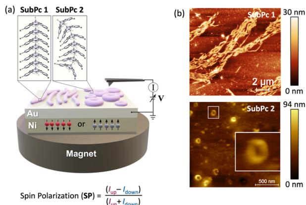
**Fig. 3** (a) Schematic illustration of the mc-AFM setup used to assess the CISS effect in this work. The pink circular and linear forms represent the experimentally observed fibers and nanorings, respectively. The magnified view illustrates a proposed head-to-tail stacking arrangement within the self-assemblies. (b) AFM images of surfaces spin-coated with self-assembled SubPcs 1 and 2.
