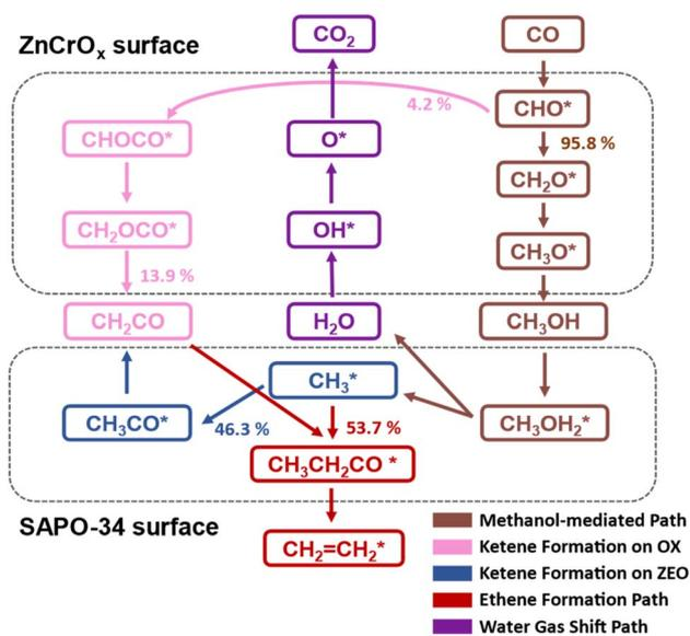
Fig. 4 Key reaction pathways extracted from the STO conversion on the  $\text{Zn}_3\text{Cr}_3\text{O}_8$ |SAPO-34 catalyst. Species on the surfaces of  $\text{ZnCrO}_x$  and SAPO-34 are enclosed in upper and lower frames, respectively. The methanol-mediated pathway is depicted in brown; the ketene formation pathways on  $\text{ZnCrO}_x$  and SAPO-34 surfaces are plotted in pink and blue, respectively; the ethene formation and water gas shift pathways are shown in red and purple, respectively.
