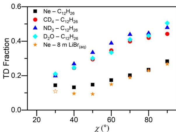
Fig. 4 TD fraction as a function of deflection angle  $\chi$  for Ne scattered from cold salty water and dodecane flat jets, and  $\text{CD}_4$ ,  $\text{ND}_3$ , and  $\text{D}_2\text{O}$  scattered from a dodecane flat jet at  $\theta_i = 60^\circ$ . Open symbols denote TD fraction values that are contaminated with beam leakage. The dodecane data are taken from ref. 62.
