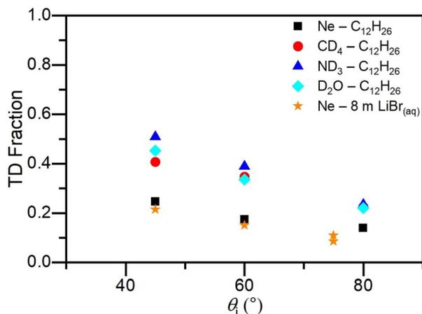
Fig. 3 TD fraction at  $\theta_f = 60^\circ$  as a function of incidence angle  $\theta_i$  for Ne scattered from cold salty water and dodecane flat jets, and  $\text{CD}_4$ ,  $\text{ND}_3$ , and  $\text{D}_2\text{O}$  scattered from a dodecane flat jet. For scattering from cold salty water at  $\theta_i = 75^\circ$ , TD fractions are plotted for  $\theta_f = 55^\circ$  and  $65^\circ$ . The dodecane data are taken from ref. 62.
