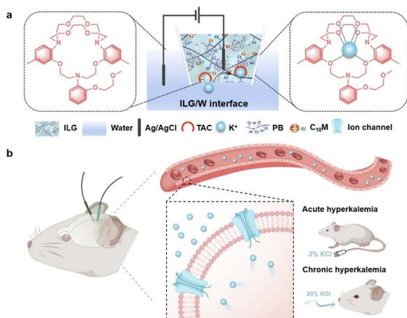
**Scheme 1** (a) Working principle of the molecularly tailored ILG-TAC/W interface supported by a micropipette for facilitating the K<sup>+</sup> transfer process. (b) *In vivo* determination of K<sup>+</sup> in the living rat brain with acute and chronic hyperkalemia models using the developed ILG-TAC electrode.
