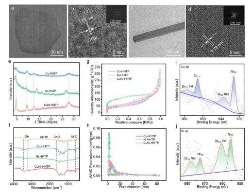
Fig. 2 The structure characterizations. (a) TEM and (b) HR-TEM images of Cu-HHTP (inset is SAED). (c) TEM and (d) HR-TEM images of Ni-HHTP (inset is SAED). (e) PXRD patterns, (f) FT-IR spectra, (g)  $N_2$  adsorption—desorption isotherms, and (h) pore-size distributions of Cu-HHTP, Ni-HHTP and CuNi-HHTP. XPS spectra of (i) Cu 2p and (j) Ni 2p of CuNi-HHTP.
