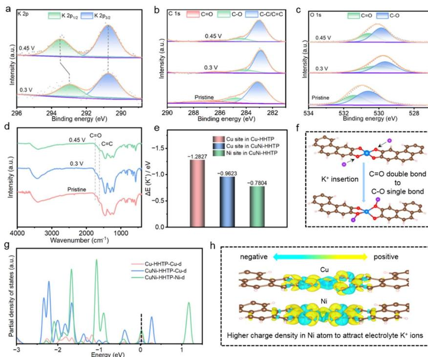
Fig. 4 Mechanism study and structural evolution of the CuNi-HHTP electrode during the charge-storage process in KCl-based electrolyte. *Ex situ* XPS spectra of (a) K 2p, (b) C 1s, (c) O 1s. (d) FT-IR spectra of the CuNi-HHTP electrode at different charging states. (e) DFT-calculated  $\Delta E_{K^+}$  of Cu-HHTP and CuNi-HHTP. (f) Illustration of  $K^+$  storage process. (g) Partial density of states and (h) the electron density difference between Cu and Ni metal centers in CuNi-HHTP.
