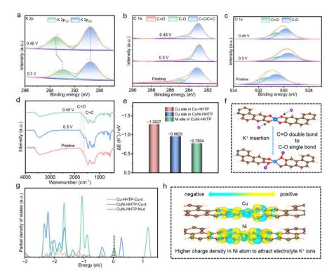
Fig. 4 Mechanism study and structural evolution of the CuNi-HHTP electrode during the charge-storage process in KCl-based electrolyte. *Ex situ* XPS spectra of (a) K 2p, (b) C 1s, (c) O 1s. (d) FT-IR spectra of the CuNi-HHTP electrode at different charging states. (e) DFT-calculated  $\Delta E_{K+}$  of Cu-HHTP and CuNi-HHTP. (f) Illustration of K<sup>+</sup> storage process. (g) Partial density of states and (h) the electron density difference between Cu and Ni metal centers in CuNi-HHTP.
