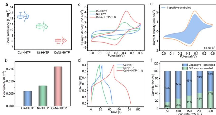
Fig. 3 The electrochemical performances. (a) Sheet resistances, (b) electrical conductivities, (c) CV curves, and (d) GCD curves of Cu-HHTP, Ni-HHTP, and CuNi-HHTP electrodes. (e) CV with capacitive-controlled contribution at  $50 \text{ mV s}^{-1}$ . (f) Contribution ratios of capacitive- and diffusion-controlled currents for the CuNi-HHTP electrode.
