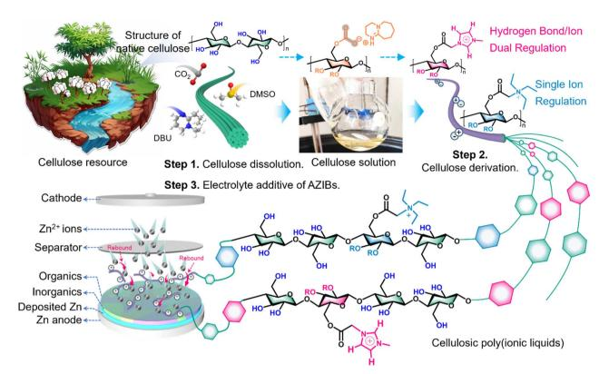
Fig. 1 Schematic diagram for the fabrication of the cellulosic PIL electrolyte additive. Step 1: dissolve cellulose in the DBU/CO<sub>2</sub>/DMSO system. Step 2: *in situ* derivatization of cellulosic PILs. Step 3: coupling hydrogen bond/ion dual regulation mechanism for highly reversible Zn anodes.
