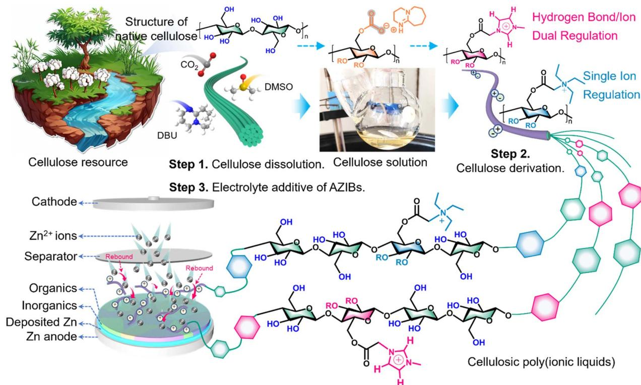
Fig. 1 Schematic diagram for the fabrication of the cellulosic PIL electrolyte additive. Step 1: dissolve cellulose in the DBU/CO<sub>2</sub>/DMSO system. Step 2: *in situ* derivatization of cellulosic PILs. Step 3: coupling hydrogen bond/ion dual regulation mechanism for highly reversible Zn anodes.
