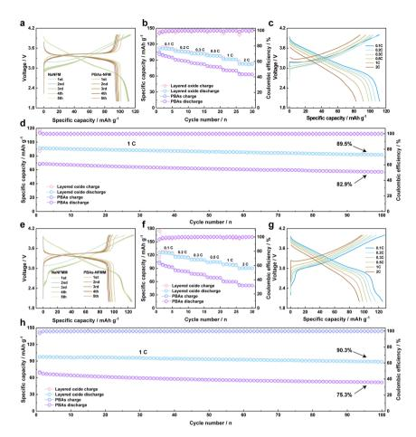
Fig. 3 Electrochemical performance within the potential window of 2–4 V: GCD curves at 0.1 C for (a) NaNFM and PBAs-NFM and (e) NaNFMM and PBAs-NFMM. Rate performance comparison of (b) NaNFM and PBAs-NFM and (f) NaNFMM and PBAs-NFMM. GCD curves at different rates of (c) NaNFM and (g) NaNFMM. Cycling performance comparison for (d) NaNFM and PBAs-NFM and (h) NaNFMM and PBAs-NFMM.
