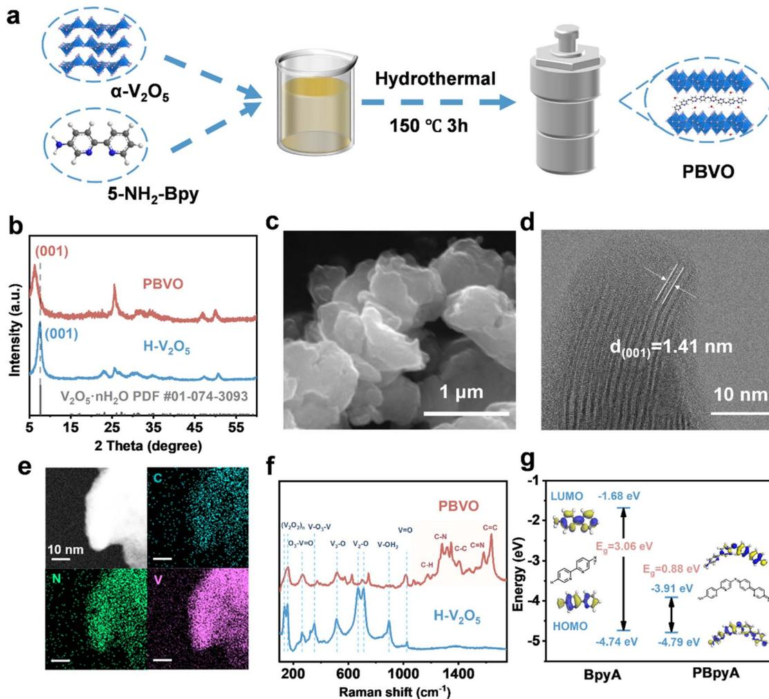
**Fig. 1** Structural and morphological characterization of PBVO. (a) Illustration of the synthesis process of PBVO; (b) XRD patterns of PBVO and H-V<sub>2</sub>O<sub>5</sub>; (c) SEM image, (d) HRTEM image, and (e) C, N and V elemental mappings of PBVO; (f) Raman spectra of PBVO and H-V<sub>2</sub>O<sub>5</sub>; (g) the highest occupied molecular orbital (HOMO) and the lowest unoccupied molecular orbital (LUMO) values of the polymer monomer (BpyA) and bipolymer (PBpyA).
