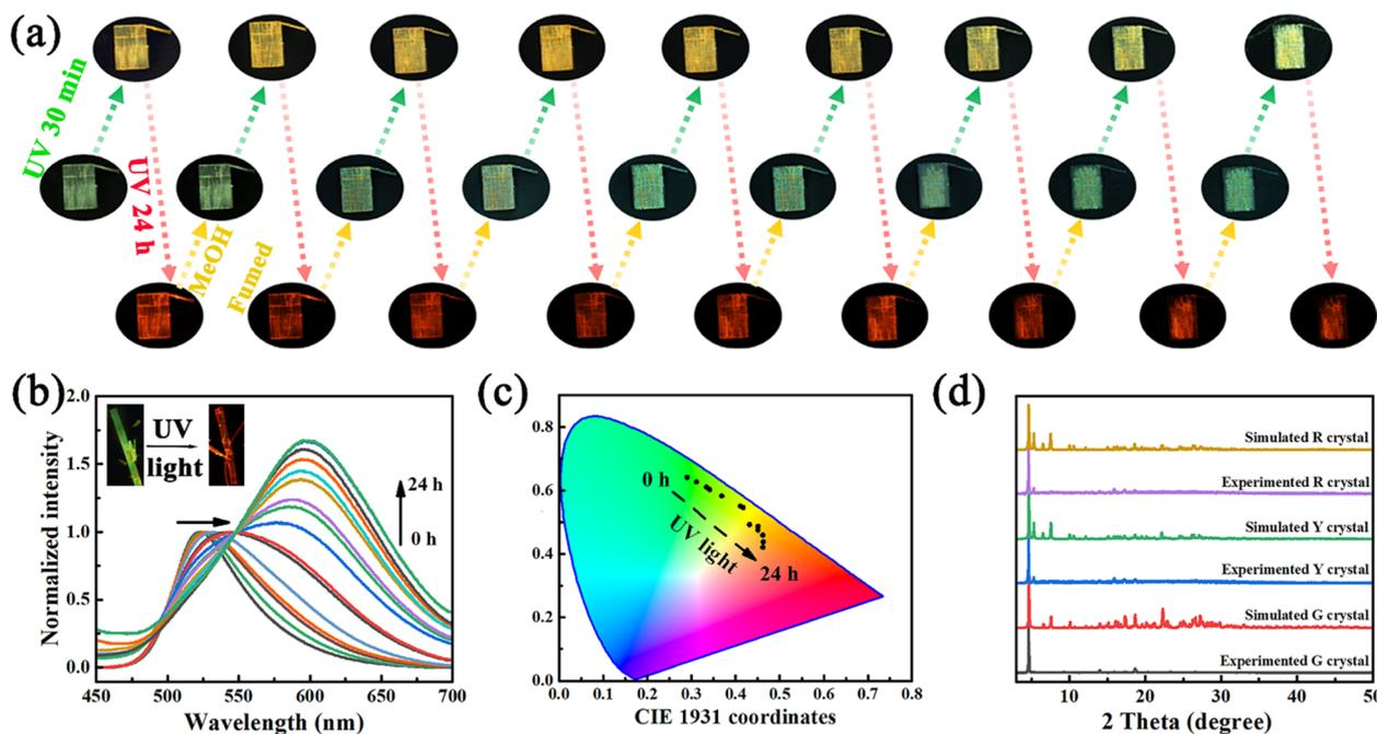
Fig. 2 (a) Photoswitchable PL images of the *p*-An-Br crystal switching 9 times between UV light irradiation and methanol fuming. (b) Fluorescence spectrum changes of crystal G with UV lamp irradiation time. (c) CIE chromaticity coordinates of crystals as a function of UV lamp irradiation time. (d) Simulated PXRD patterns of three single crystals of *p*-An-Br.
