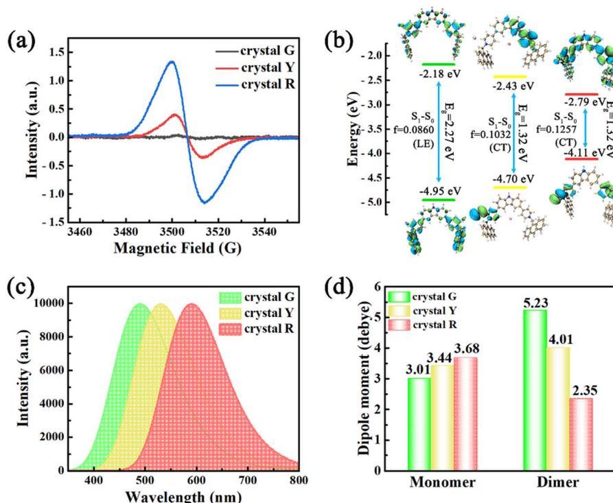
Fig. 4 (a) EPR spectra of the three crystals of *p*-An-Br. (b) Electron distribution and energy levels of molecular orbitals of the three crystals. (c) Calculated fluorescence emission spectra of the three types of crystals. (d) Dipole moment of the three crystals calculated from DFT calculations in monomer and dimer states.
