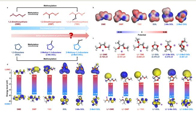
Fig. 1 (a) Schematic diagram of the molecular design of weakly solvated chain ethers and cyclic ethers. (b) ESP maps of various ether solvent molecules. (c) Bonding energy of Li<sup>+</sup> with different ether solvent molecules. (d) HOMO-LUMO levels of different solvent molecules and aggregates bound to Li<sup>+</sup>.
