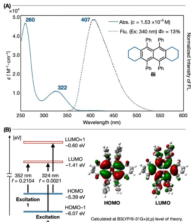
Fig. 4 (A) UV-vis absorption and emission spectra of **8i** ( $c = 1.53 \times 10^{-5}$  M) in THF. Excitation light was 340 nm. (B) Possible transitions calculated by TD-DFT at the B3LYP/6-31G+(d,p) level of theory and depiction of frontier MOs.
