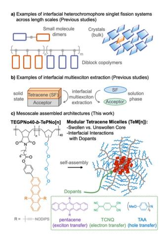
Fig. 1 (a) Conventional architectures comprising two types of singlet fission chromophores. (b) Examples of solid-state and solution phase designs to investigate multiexciton generation and exciton/charge transfer mechanisms at heterointerfaces (bilayers and collisions). (c) Macromolecular approach to access mesoscale structures (e.g. micelles) that can be readily doped with solvents to induce chain mobility of the hydrophobic core, as well as exciton/charge donors and acceptors.
