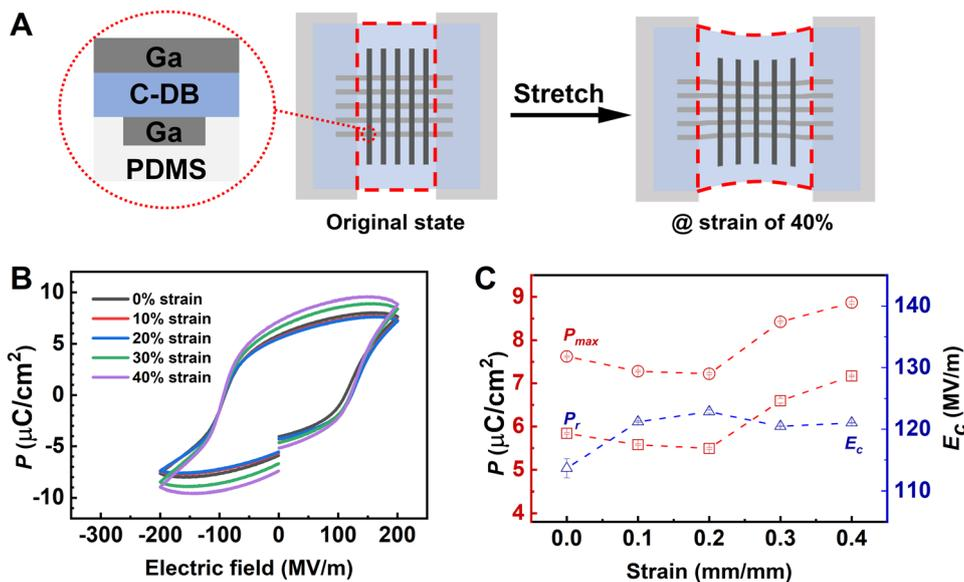
Fig. 6 Ferroelectric response of the elastic films under strain. (A) Schematic structure of the elastic device in the stretching setup under 0–40% strain. (B)  $P$ – $E$  loops at 1 kHz under 0–40% strain. (C)  $P_r$ ,  $P_{max}$ , and  $E_c$  under different strains.
