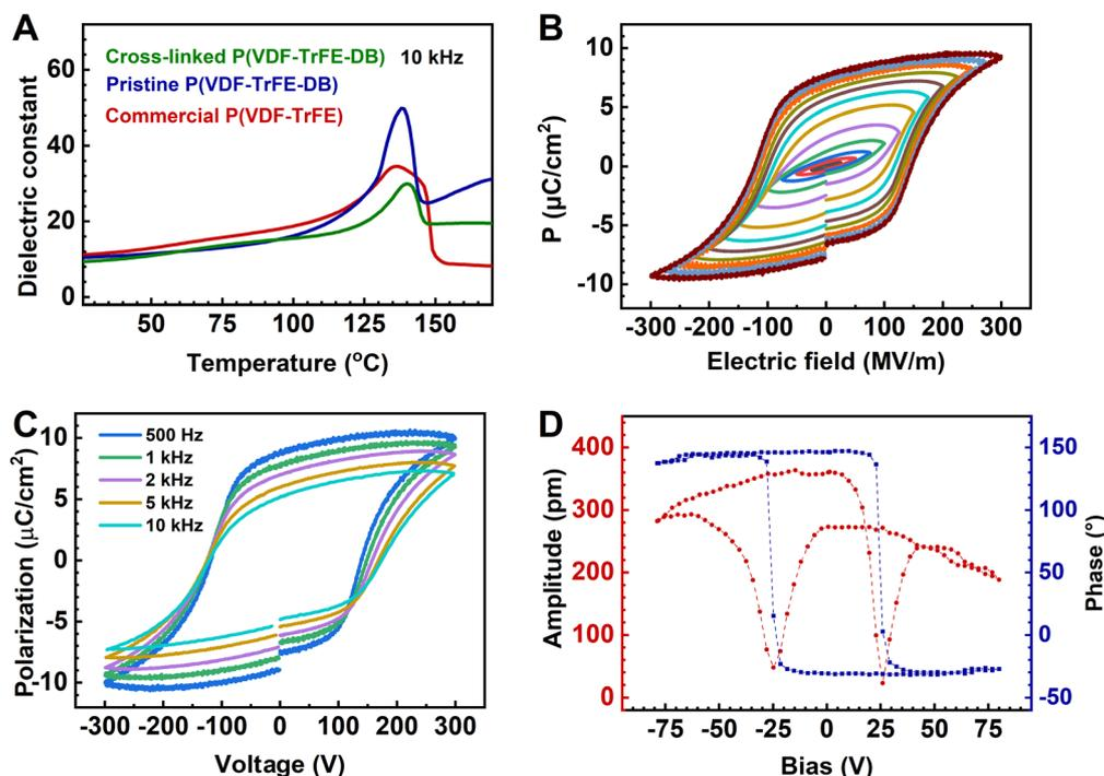
Fig. 5 Ferroelectric properties of the crosslinked P(VDF-TrFE-DB) films. (A)  $\epsilon-T$  curves of P(VDF-TrFE) 80/20 mol%, pristine P(VDF-TrFE-DB) and crosslinked P(VDF-TrFE-DB) films at 10 kHz. (B and C)  $P-E$  loops of Au/crosslinked P(VDF-TrFE-DB)/Au under different electric fields at 1 kHz (B) and at different frequencies (C). (D) Phase–voltage hysteresis and amplitude–voltage butterfly loop from PFM measurements.
