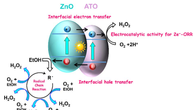
Scheme 1 Schematic description of the action mechanism of ATO-CL/ZnO photocatalysis for the production of \text{H}_2\text{O}_2 from ethanol aqueous solution.
