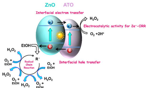
Scheme 1 Schematic description of the action mechanism of ATO-CL/ZnO photocatalysis for the production of \text{H}_2\text{O}_2 from ethanol aqueous solution.
