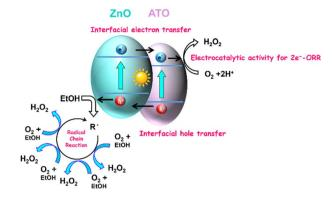
Scheme 1 Schematic description of the action mechanism of ATO-CL/ZnO photocatalysis for the production of  $H_2O_2$  from ethanol aqueous solution.
