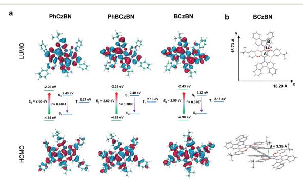
Fig. 1 (a) Theoretical calculated results of PhCzBN, PhBCzBN, and BCzBN (DFT and TD-DFT were performed based on the B3LYP density functional method with the basis set 6-31G(d, p); the S1 and T1 energy values were calculated by SCS-CC2 using the MRCC Program with the cc-PVDZ method). (b) Single-crystal structure of BCzBN and its stacking model.
