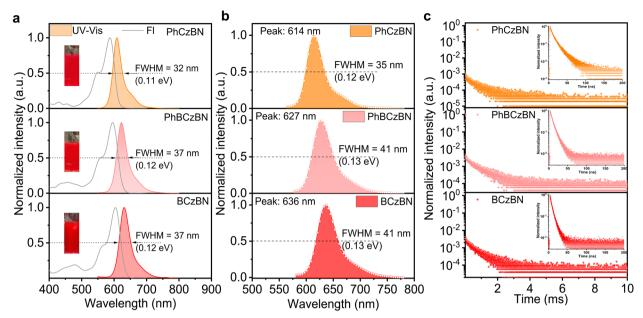
Fig. 2 (a) UV-visible absorption (UV-vis) and fluorescence (Fl.) spectra of PhCzBN, PhBCzBN, and BCzBN in toluene ( $1 \times 10^{-5}$  mol L<sup>-1</sup>) at 300 K. (b) Fl. spectra measured in DMIC-TRZ film. (c) Transient photoluminescence spectra recorded in DMIC-TRZ film.
