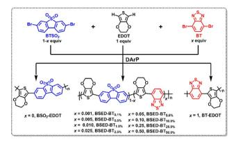
Scheme 1 Synthetic routes of bi-polymers BSO<sub>2</sub>-EDOT and BT-EDOT and terpolymer BSED-BT<sub>x</sub> (x represents the molar ratio of BT) via DArP polymerization.
