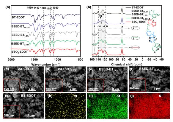
Fig. 1 (a) FT-IR spectra and (b) solid-state  $^{13}$ C NMR spectra of BSO<sub>2</sub>-EDOT, BSED-BT<sub>0.5%</sub>, BSED-BT<sub>1.0%</sub>, BSED-BT<sub>50.0%</sub>, and BT-EDOT; SEM images of (c) BSO<sub>2</sub>-EDOT, (d) BSED-BT<sub>0.5%</sub>, (e) BSED-BT<sub>1.00%</sub>, (f) BSED-BT<sub>50.0%</sub>, and (g) BT-EDOT. EDS elemental mapping of (h) N, (i) O and (j) S in BSED-BT<sub>0.5%</sub>.
