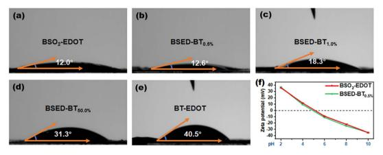
Fig. 5 Water CAs of BSO<sub>2</sub>-EDOT (a), BSED-BT<sub>0.5%</sub> (b), BSED-BT<sub>1.0%</sub> (c), BSED-BT<sub>50.0%</sub> (d), and BT-EDOT (e); (f) zeta potentials of BSO<sub>2</sub>-EDOT and BSED-BT<sub>0.5%</sub>.
