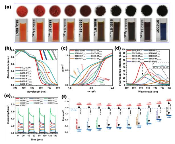
Fig. 2 (a) Photographs of all polymers. (b) UV-vis DRS and (c) Tauc-plot of  $BSO_2$ -EDOT, BSED-BT<sub>0.1%</sub>, BSED-BT<sub>0.5%</sub>, BSED-BT<sub>0.5%</sub>, BSED-BT<sub>0.5%</sub>, BSED-BT<sub>0.5%</sub>, and BSED-BT<sub>0.5%</sub>, (d) Steady state PL spectra, (e) energy band diagrams and (f) transient photocurrents under visible light irradiation of all polymers.
