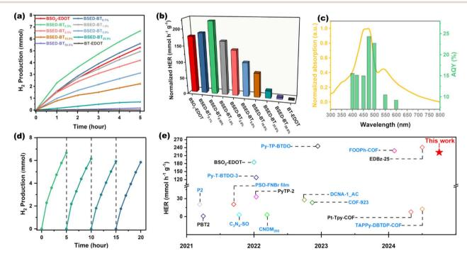
Fig. 3 (a) PHP as a function of time for 6 mg polymers under visible light irradiation. (b) Normalized hydrogenolysis reaction rates of all polymers. (c) AQYs of PHP for BSED $-BT_{0.5\%}$  at six different incident light wavelengths. (d) Cycling stability test for BSED $-BT_{0.5\%}$ . (e) Comparison of the HER of BSED $-BT_{0.5\%}$  with those of other recently reported photocatalysts (blue colour indicates that the HER added Pt as a co-catalyst). <sup>28,35,38,45-56</sup>
