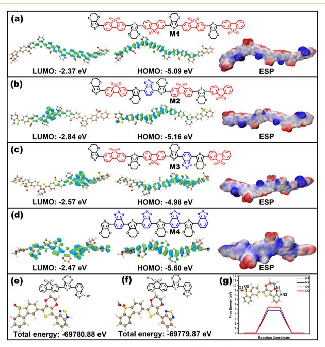
Fig. 6 DFT-predicated FMO distributions and ESPs of the tetramers M1 (a), M2 (b), M3 (c), and M4 (d); the total energy of protons adsorbed on BT (e) and on BTSO<sub>2</sub> (f); the adsorption free energy during  $H^+$  reduction (g).
