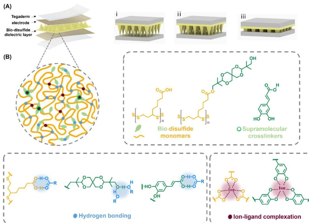
Fig. 1 Graphical illustrations of the micropyramid-structured dynamic poly(disulfide)-based capacitive pressure sensor. (A) Conceptual illustrations of the dynamic disulfide polymer-based wearable capacitive pressure sensor and its physical appearance distortion upon different external pressures. (B) Graphical illustrations of the chemical composition of the micropyramid dielectric dynamic polymer.
