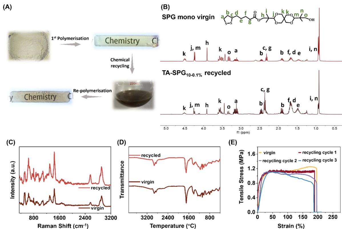
Fig. 4 TA-SPG<sub>10-0.1%</sub> closed-loop recycling assessment. (A) Graphic illustrations of the closed-loop solvolytic recycling. The comparisons of (B) <sup>1</sup>H Nuclear Magnetic Resonance (<sup>1</sup>H NMR) spectra of the TA-SPG monomeric precursor. (C) Raman spectra. (D) FTIR spectra and (E) tensile stress-strain curves of virgin/recycled TA-SPG<sub>10-0.1%</sub>.
