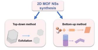
Scheme 1 Synthesis process of 2D MOF nanosheets
