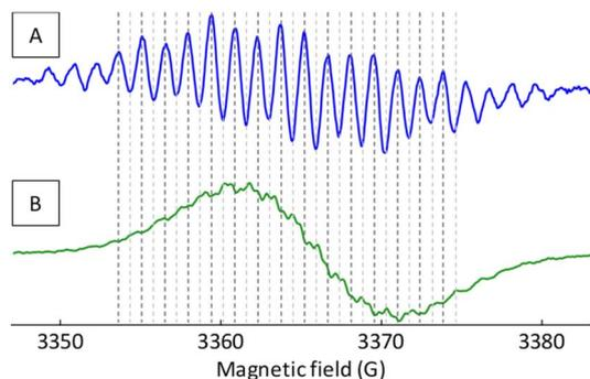
Fig. 3 ESR spectra recorded at RT after electrochemical reduction of  $2(\text{PF}_6)_4$  in DMF,  $n\text{Bu}_4\text{NPF}_6$  0.1 M at  $E_{\text{app}} = -1$  V, (A) spectrum recorded after addition of  $2e^-$  per molecule, (B) spectrum recorded after addition of  $1e^-$  per molecule.
