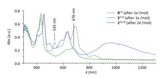
Fig. 4 UV/Vis/NIR (l = 1 mm) spectra of the reduced species of  $8^{2+}$  (1 mM) and  $2^{4+}$  (0.5 mM) in DMF ( $nBu_4NPF_6$  0.1 M)
