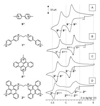
Fig. 1 CV curves (DMF, nBu<sub>4</sub>NPF<sub>6</sub> 0.1 M, VC  $\emptyset$  = 3 mm, E vs. Ag<sup>+</sup>/Ag, 100 mV s<sup>-1</sup>) of (A)  $9^{2+}$  (1 mM), (B)  $1^{4+}$  (0.5 mM), (C)  $8^{4+}$  (1 mM) and (D)  $2^{4+}$  (0.5 mM).
