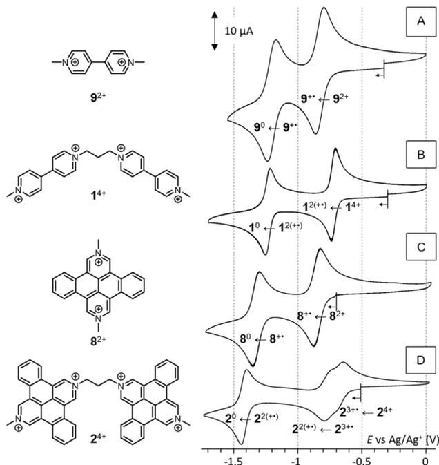
Fig. 1 CV curves (DMF,  $n\text{Bu}_4\text{NPF}_6$  0.1 M, VC  $\varnothing = 3$  mm,  $E$  vs.  $\text{Ag}^+/\text{Ag}$ ,  $100 \text{ mV s}^{-1}$ ) of (A)  $9^{2+}$  (1 mM), (B)  $1^{4+}$  (0.5 mM), (C)  $8^{2+}$  (1 mM) and (D)  $2^{4+}$  (0.5 mM).
