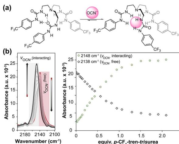
Fig. 3 (a) Binding scheme and (b) *in situ* FTIR titration of *p*-CF<sub>3</sub>-tren-tris(urea) (12.7 mM) into TBAOCN in anhydrous 20% DMSO in MeCN at 298 K.
