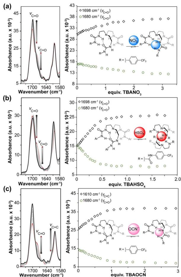
Fig. 2 *In situ* FTIR titration spectra (left) and plot of absorbance changes (right) for *p*-CF<sub>3</sub>-tren-tris(urea) with (a) TBANO<sub>3</sub>, (b) TBAHSO<sub>4</sub>, and (c) TBAOCN in anhydrous 20% DMSO in MeCN at 298 K.
