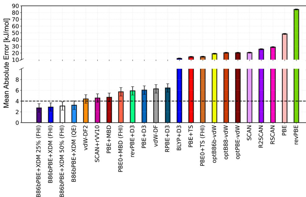
Fig. 5 Benchmark of DFT functionals against reference DMC values<sup>30</sup> on the lattice energies of the X23 dataset. The functionals are listed from left to right in order of decreasing performance (higher MAE). The reported error bar is the average statistical error bar of the DMC reference values. "QE" and "FHI" mean that the number have been respectively computed with Quantum Espresso<sup>105</sup> or FHI-aims.<sup>106</sup>
