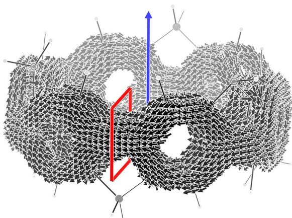
Fig. 5 HOMO contribution to the electron current density induced in **2** by a magnetic field parallel to the main symmetry axis (blue arrow). The current lower than 0.04 a.u. are not shown. Maximum current is 0.34 a.u. Red square delimits the integration region for the calculation of aryl-aryl bond current strength.
