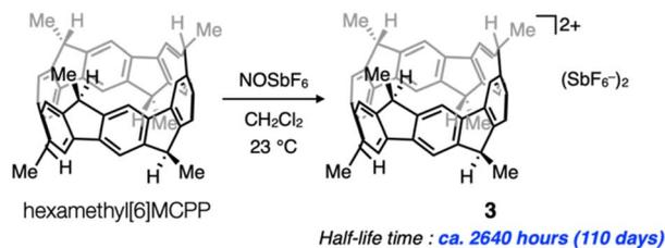
**Scheme 2** Chemical oxidation of hexamethyl[6]MCPP. Reaction conditions: hexamethyl[6]MCPP (7.6  $\mu\text{mol}$ , 4.6 mg, 1.0 equiv.),  $\text{NOSbF}_6$  (23  $\mu\text{mol}$ , 6.0 mg, 3.0 equiv.),  $\text{CH}_2\text{Cl}_2$  (3.0 mL). Half-life time was elucidated in  $\text{CH}_2\text{Cl}_2$  solution at 23  $^\circ\text{C}$  under air.
