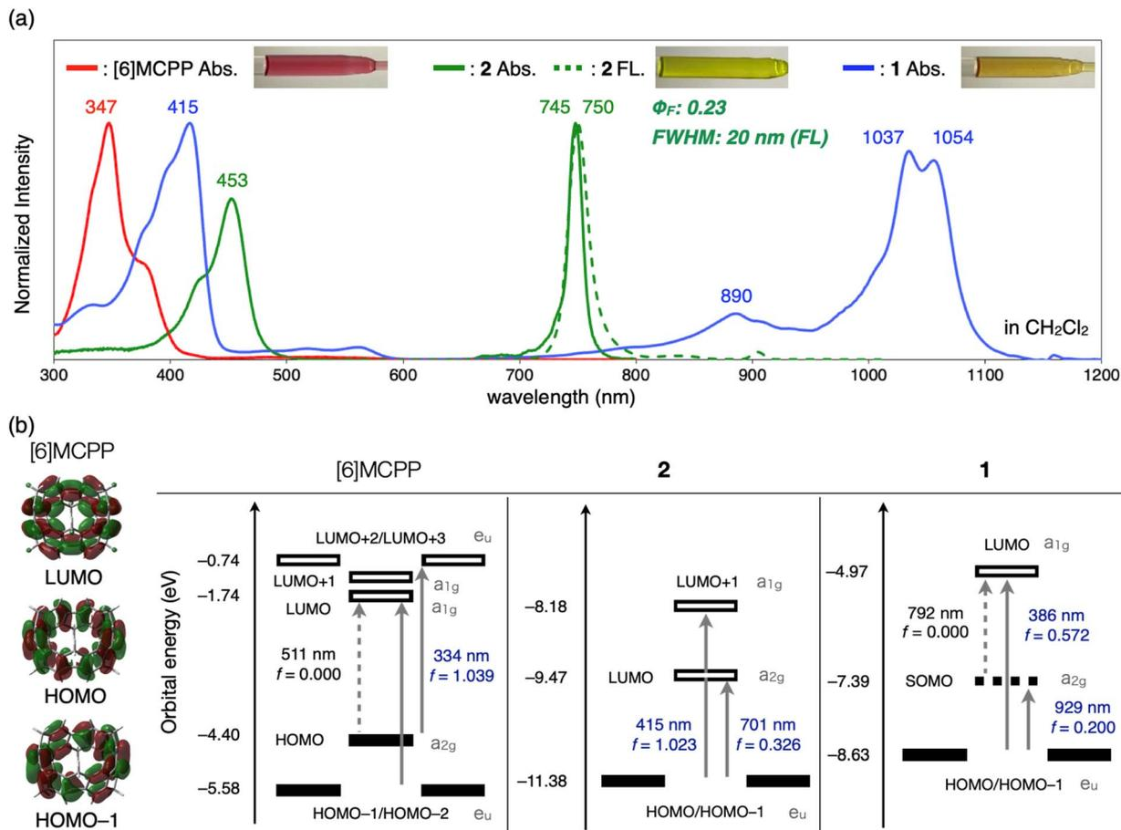
Fig. 3 (a) UV-vis-NIR absorption (solid line) and fluorescence (dashed line) spectra of  $\text{CH}_2\text{Cl}_2$  solutions of [6]MCP, 1, and 2. Fluorescence spectrum of 2 was recorded upon excitation at 450 nm. (b) Frontier molecular orbitals of [6]MCP and transitions estimated by TDDFT calculation.
