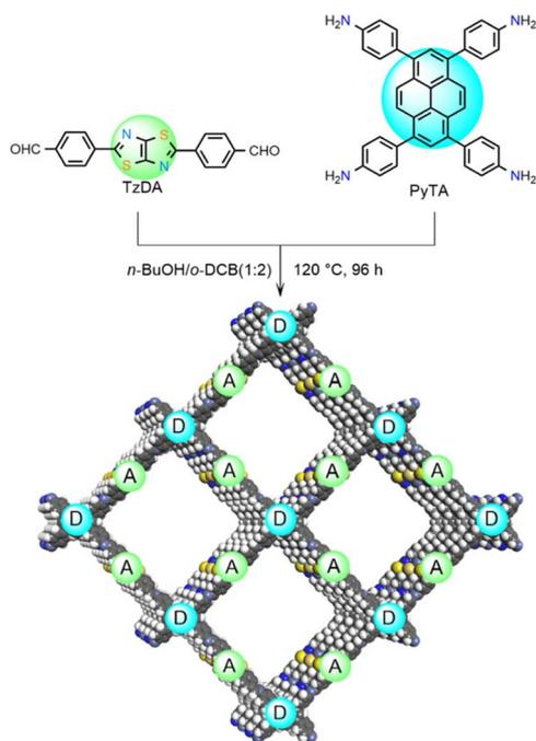
Fig. 6 Synthesis of PyTz-COF under solvothermal conditions. Reproduced from ref. 86 with permission from John Wiley and Sons, copyright 2020.
