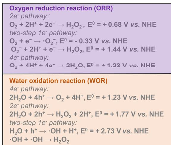
Fig. 14 Mechanism diagram of photocatalytic production of H<sub>2</sub>O<sub>2</sub>.
