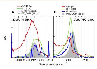
Fig. 9 Evolution-associated difference absorption spectra and time constants obtained from a global analysis of the time-resolved IR absorption data measured with (A) DMA-PT-DMA and (B) DMA-PTO-DMA in DMSO assuming a series of successive exponential steps and last spectra obtained with the single branch analogues (grey).
