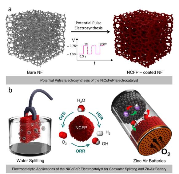
Fig. 1 Schematic illustration of the electrosynthesis of the NCFP electrocatalyst and its applications. (a) Electrosynthesis of the NCFP electrocatalyst that lasts for just 2 min (see inset) (b) illustration of the practical application of the multifunctional NCFP electrocatalyst for overall (sea) water splitting and zinc-air batteries.
