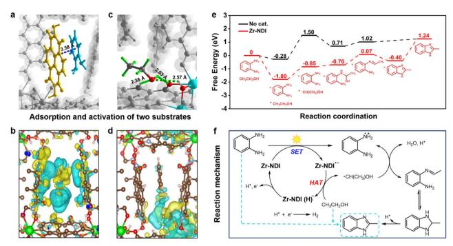
Fig. 5 The DFT calculation and proposed reaction mechanism. (a) Optimized structure of OPD in the Zr-NDI pores. (b) Diagram of the charge density difference between OPD and Zr-NDI. (c) Optimized structure of ethanol in the Zr-NDI pores. (d) Diagram of the charge density difference between ethanol and Zr-NDI. (e) Free energy diagram for cross-coupling of OPD and ethanol to 2MBZ with or without catalyst. (f) Proposed reaction mechanism for photocatalytic 2MBZ synthesis over Zr-NDI.
