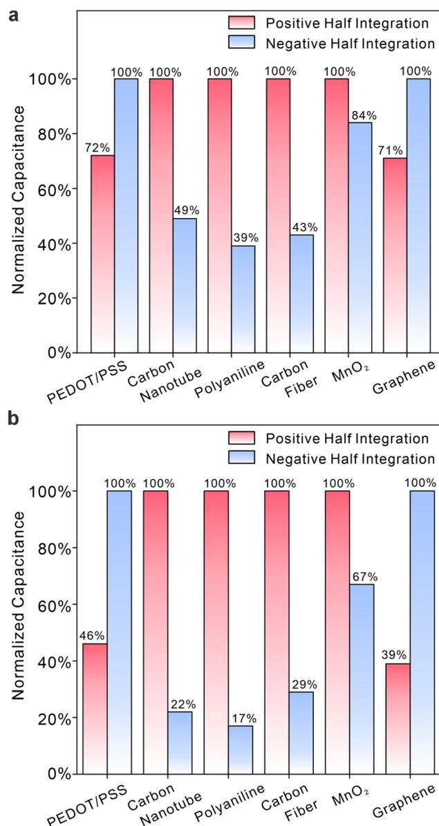
Fig. 4 (a and b) A comparison of normalized charge between positive and negative overpotentials (*versus*  $E_{ocp}$ ) for six different materials with (a) and without (b) membranes in 0.1 M NaCl solutions. Blue bars represent the normalized amount of charge storage under negative potentials and red bars denote the normalized amount of charge storage under positive potentials.
