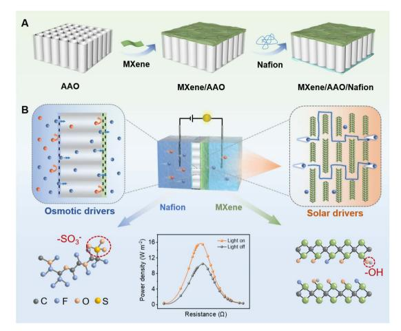
Scheme 1 Schematic illustration of the two-sided asymmetric MXene/AAO/Nafion membrane for osmotic energy harvesting. (A) Fabrication process of the MXene/AAO/Nafion membrane. (B) High-efficiency osmotic energy harvesting using the two-sided asymmetric MXene/AAO/Nafion membrane. Orange and blue arrows indicate the transport directions of anions and cations, respectively.
