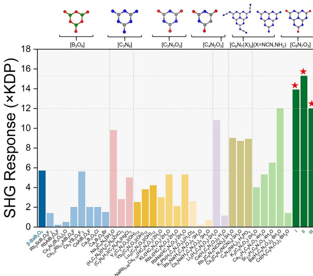
Fig. 4 SHG response of the compounds containing six-member ring  $\text{B}_3\text{O}_6$ -type  $\pi$ -conjugated groups and large  $\text{C}_6\text{N}_7$ -type  $\pi$ -conjugated groups.
