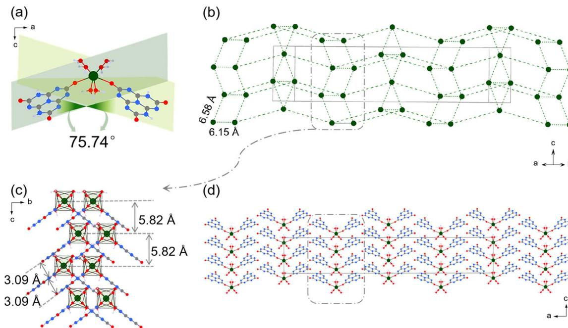
Fig. 1 (a) The coordination environment of  $\text{Gd}^{3+}$ ; (b) the stacking diagram of  $\text{Gd}^{3+}$  cations; (c) the stacking pattern of  $\text{Gd}^{3+}$  polyhedra; and (d) the crystal structure of II. The olive-green, red, gray, blue, and light gray balls represent Gd, O, C, N, and H, respectively.
