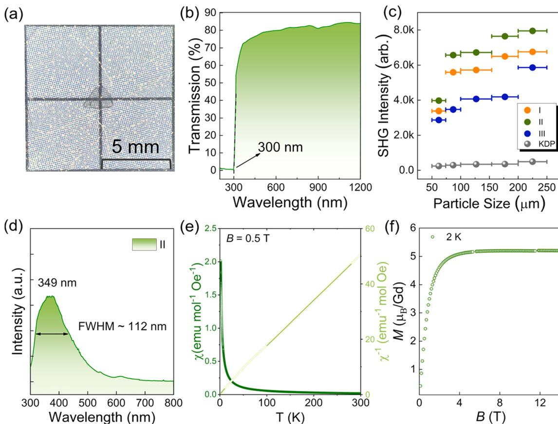
Fig. 2 (a) The grown crystal of II. (b) UV-vis-NIR transmittance spectrum of II. (c) SHG measurements of the three compounds. (d) Photoluminescent measurements of II. (e)  $\chi$  versus temperature of II for FC data (green symbol line) and the plot of  $1/\chi$  versus temperature (light green symbol line). (f) Magnetic susceptibility as a function of the applied field for the II samples with Gd.
