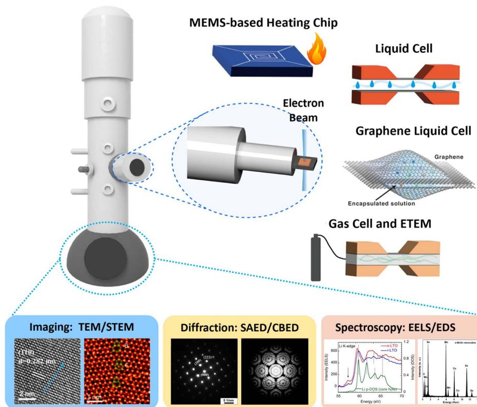
Fig. 2 Schematics of TEM and *in situ* chips and cells fabricated by MEMS. Reproduced with permission.<sup>43–46</sup> Copyright 2013, Elsevier. Copyright 2024, Elsevier. Copyright 2016, American Chemical Society. Copyright 2019, American Chemical Society.
