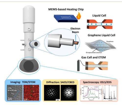
Fig. 2 Schematics of TEM and *in situ* chips and cells fabricated by MEMS. Reproduced with permission. 43–46 Copyright 2013, Elsevier. Copyright 2014, Elsevier. Copyright 2016, American Chemical Society. Copyright 2019, American Chemical Society.
