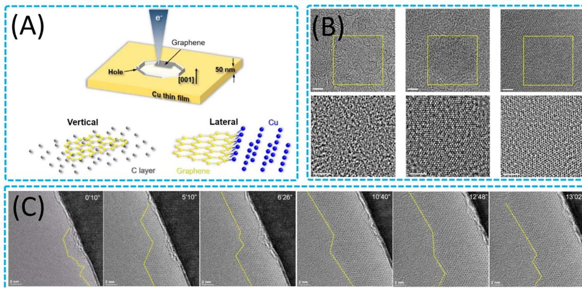
Fig. 12 Growth of 2D nanomaterials through gas–solid interactions. (A) ETEM experimental setup and typical observations of *in situ* graphene growth. (B) Nucleation and growth of graphene from an amorphous C layer. (C) Time-resolved HRTEM images showing the lateral epitaxial growth of graphene on the Cu edge. Reproduced with permission.<sup>230</sup> Copyright 2020, American Chemical Society.
