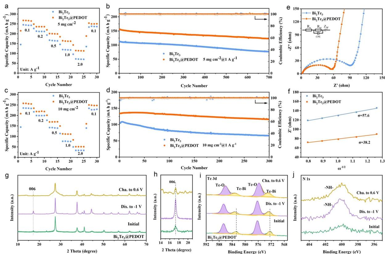
Fig. 4 (a) Rate performances and (b) cycle life of  $Bi_2Te_3$  and  $Bi_2Te_3@PEDOT$  ( $5\text{ mg cm}^{-2}$ ) at  $1\text{ A g}^{-1}$ . (c) Rate capabilities and (d) cycle life of  $Bi_2Te_3$  and  $Bi_2Te_3@PEDOT$  ( $10\text{ mg cm}^{-2}$ ) at  $1\text{ A g}^{-1}$ . (e) EIS spectra and (f) relationship between  $Z'$  and  $\omega^{-1/2}$  of  $Bi_2Te_3$  and  $Bi_2Te_3@PEDOT$ . (g and h) *Ex situ* XRD patterns, (i) Te 3d XPS spectra, and (j) N 1s XPS spectra of  $Bi_2Te_3@PEDOT$ .
