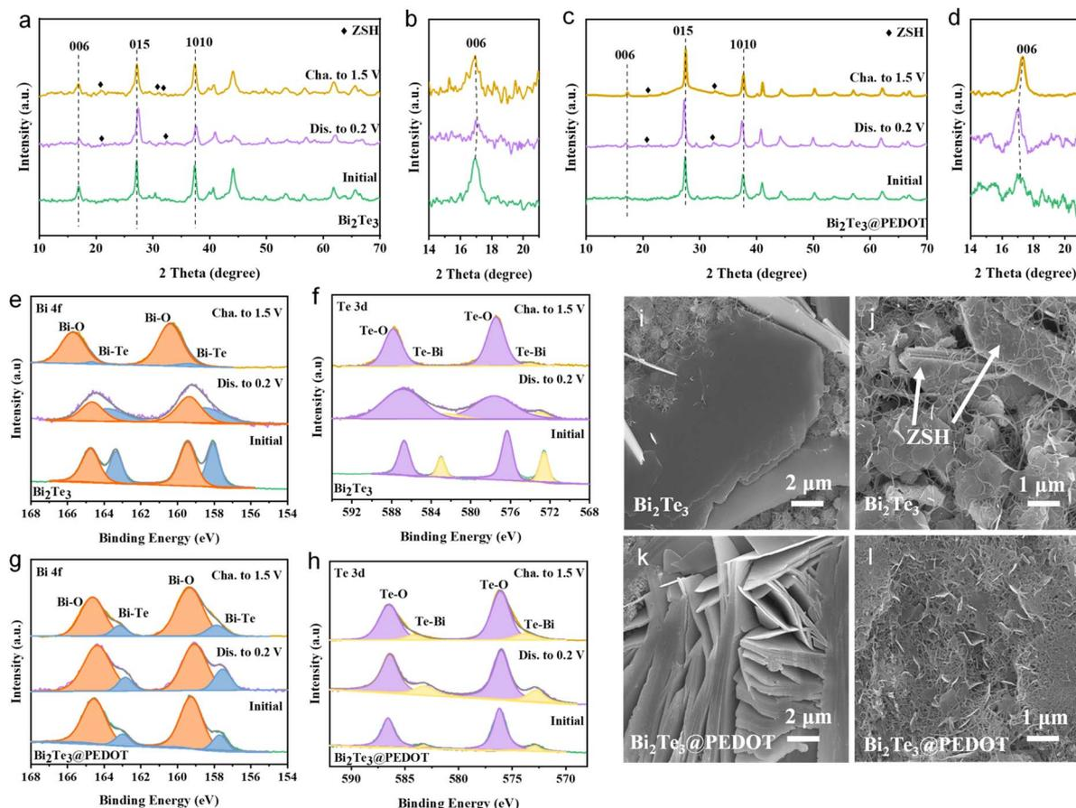
Fig. 3 (a–d) *Ex situ* XRD patterns, (e and g) Bi 4f XPS spectra, and (f and h) Te 3d XPS spectra of  $\text{Bi}_2\text{Te}_3$  and  $\text{Bi}_2\text{Te}_3@\text{PEDOT}$ . SEM images of (i and j)  $\text{Bi}_2\text{Te}_3$  and (k and l)  $\text{Bi}_2\text{Te}_3@\text{PEDOT}$  at the fully discharged/charged states.
