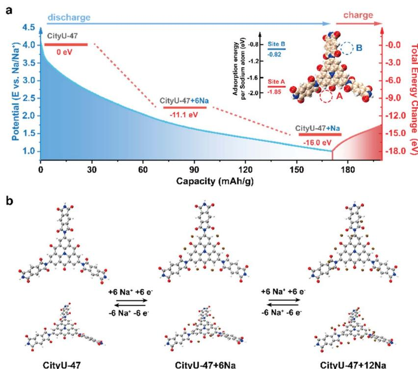
Fig. 6 DFT calculations. (a) Proposed sodiation pathway of the CityU-47 electrode, with redox potential vs. Na/Na<sup>+</sup> on the left axis and total energy change on the right axis. (b) The corresponding structural evolution of CityU-47 during the sodiation procedure.
