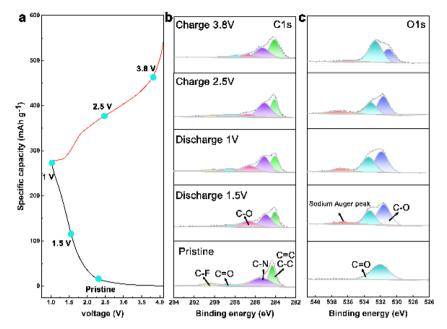
Mechanistic behavior of CityU-47. (a) Charge-discharge curves. (b and c) Ex situ XPS spectra of C 1s and O 1s.
