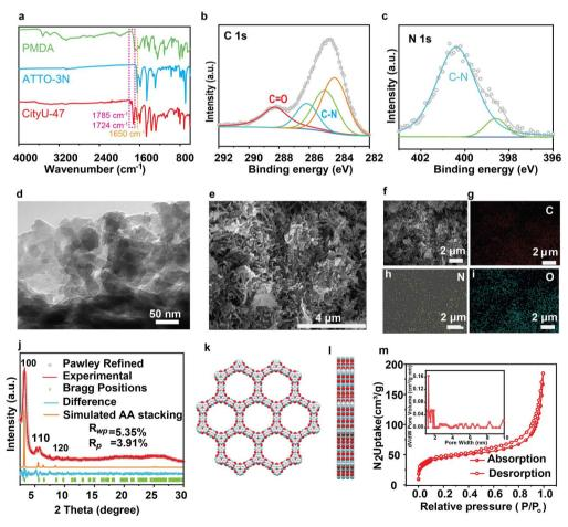
Fig. 2 Structural characterizations of CityU-47. (a) FTIR spectra of CityU-47 and starting materials. XPS profiles of CityU-47: (b) C 1s and (c) N 1s. (d) TEM images, and (e) SEM images. (f–i) EDX mapping images of C, N, and O. (j) PXRD patterns of experimental (red), Pawley-refined (grey), and simulated stacking (orange) results, and their difference (light blue), and Bragg positions (green). (k and l) Space-filling model of AA stacking. (m) Nitrogen adsorption—desorption isothermsat 77 K.
