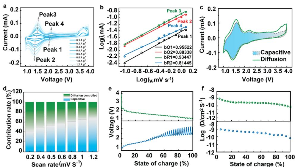
Fig. 4 Kinetic tests of CityU-47. (a) CV curves at various scan rates. (b) Plots of the *b* value at different peak rates. (c) The capacitive contribution of the CV curves. (d) The capacitive contribution with the proportions at different scan rates. (e) GITT curves of charging and discharging. (f) The corresponding  $D_{\text{Na}^+}$  for GITT.
