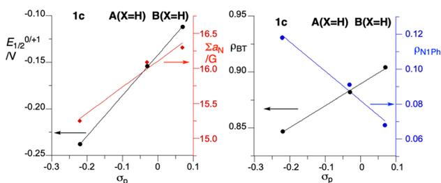
Fig. 13 Left: correlation of  $E_{1/2}^{0/+1}$  (black) and the sum of  $hfcc$   $a_{\text{N}}$  for the triazine ring (red) with Hammett parameters  $\sigma_p$  for -SPh (0.07), -OPh, (-0.03) and -NPh<sub>2</sub>, (-0.22). Right: correlation of DFT spin density for the benzo[e][1,2,4]triazine ring ( $\rho_{\text{BT}}$ , black) and for the benzene ring at the N(1) position of the triazine ( $\rho_{\text{N1Ph}}$ , blue) with  $\sigma_p$ .
