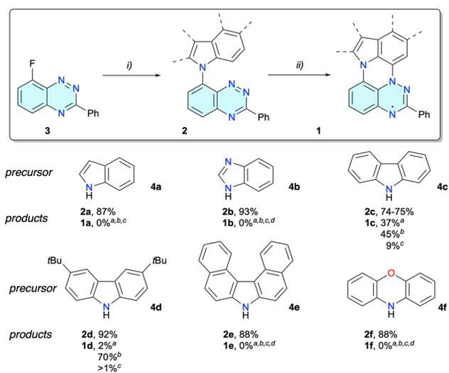
Scheme 1 Synthesis of benzo[*e*][1,2,4]triazines **2** and their photocyclization to radicals **1** at  $c \approx 1$  mM. <sup>a</sup> Reagents and conditions: (i) heteroarene **4a–4f**, 60% NaH, dry DMSO, 80 °C, 3 h; (ii) 300 W halogen lamp in a Pyrex flask, 1 mM (a) in CH<sub>2</sub>Cl<sub>2</sub>, (b) in EtOAc or (c) in EtOH, 30–35 °C, 72 h; (d) no reaction.
