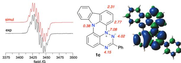
Fig. 14 Left: Experimental (black) and simulated (red) EPR spectra for **1c** recorded in benzene at ca. 20 °C. Right: assignment of the resulting  $hfcc$  (G) and the total spin density in **1c** based on DFT calculations in benzene dielectric medium. Contour values are plotted at  $\pm 0.02$  ( $e/\text{bohr}^3$ )<sup>1/2</sup>.
