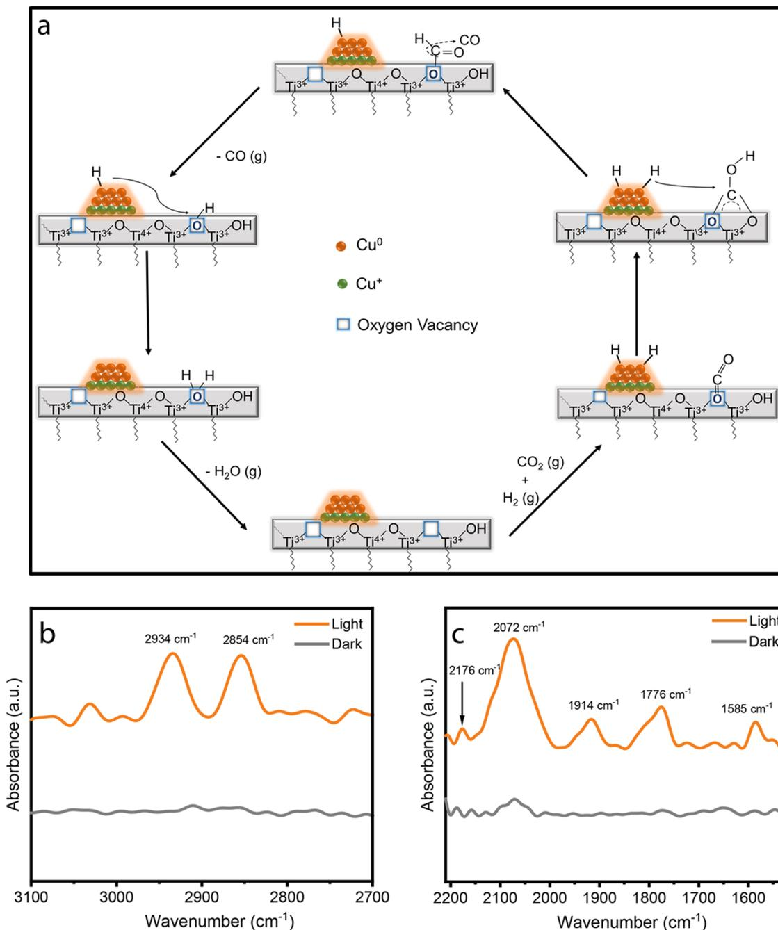
Fig. 7 Molecular mechanism of  $\text{CO}_2$  reduction. (a) Proposed reaction mechanism for  $\text{CO}_2$  reduction over DFNS/ $\text{TiO}_2$ -Cu10; (b) and (c) *in situ* DRIFTS spectra for DFNS/ $\text{TiO}_2$ -Cu10 under  $\text{CO}_2 + \text{H}_2$  environment in light and dark conditions.
