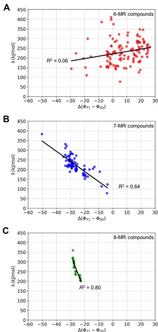
Fig. 7 Reorganization energies ( $\lambda$ ) plotted against the differences in average dihedral angles between the  $S_0$  and  $T_1$  states ( $\Delta(\phi_{T_1} - \phi_{S_0})$ ) as a measure of the change in puckering for (A) 6-, (B) 7-, and (C) 8-MR compounds.  $\lambda$  and  $\Delta(\phi_{T_1} - \phi_{S_0})$  are computed at the M06-2X/6-311G(d,p) level.
