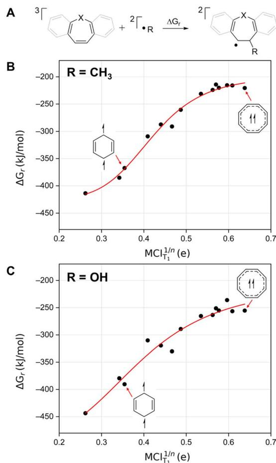
Fig. 3 (A) Schematic depiction for the reaction of radicals with various species. Reaction energies as a function of the  $T_1$  state (anti)aromatic character of the  $(6\pi)8\pi$ -electron cycle as assessed through the  $MCI_{T_1}$  values for (B) methyl radical and (C) hydroxyl radical. For simplicity, only benzene and COT were shown, see Fig. S2† for the labelled plot. For unsymmetric structures containing heteroatoms, the methyl group was added to the furthest carbon from the heteroatom.
