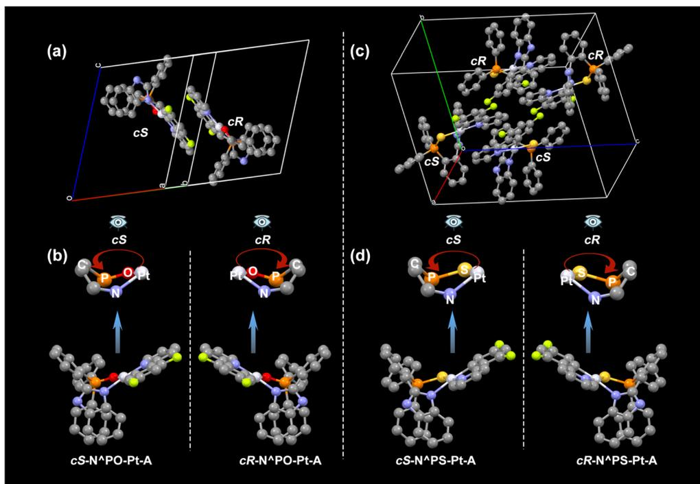
Fig. 6 X-ray single-crystal structures of *rac*-N<sup>A</sup>PO-Pt-A: (a) one crystal cell and (b) *cR*-N<sup>A</sup>PO-Pt-A and *cS*-N<sup>A</sup>PO-Pt-A molecular structures and the definition of (*cR*)/(*cS*) chirality (some atoms are omitted); X-ray single-crystal structures of *rac*-N<sup>A</sup>PS-Pt-A: (c) one crystal cell and (d) *cR*-N<sup>A</sup>PS-Pt-A and *cS*-N<sup>A</sup>PS-Pt-A molecular structures and the definition of (*cR*)/(*cS*) chirality (some atoms are omitted).
