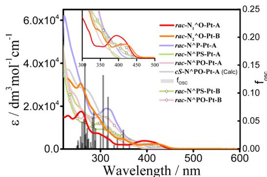
Fig. 3 Experimental absorption spectra of Pt(II) complexes in CH<sub>2</sub>Cl<sub>2</sub> solution ( $5.0 \times 10^{-5}$  mol dm<sup>-3</sup>).
