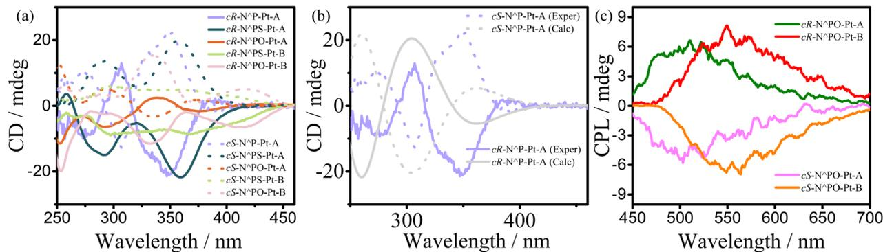
Fig. 9 (a) CD spectra of Pt(II) complexes in dilute  $\text{CH}_2\text{Cl}_2$  solution ( $3.0 \times 10^{-5} \text{ mol dm}^{-3}$ ); (b) experimental and calculated CD spectra of cR/cS-N<sup>o</sup>P-Pt-A complexes in dilute  $\text{CH}_2\text{Cl}_2$  solution; (c) CPL spectra of Pt(II) complexes in powder.
