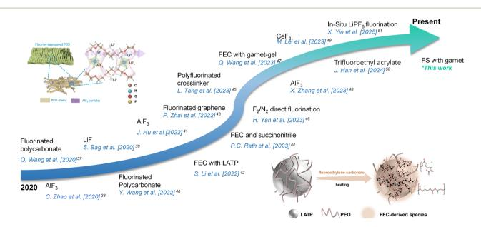
Scheme 1 Recent literature reports on various interfacial engineering using fluorine-based modifications for solid-state lithium metal batteries. Adapted with permission from [ref. 41] Copyright 2022 Springer Nature and [ref. 42] Copyright 2022 American Chemical Society.
